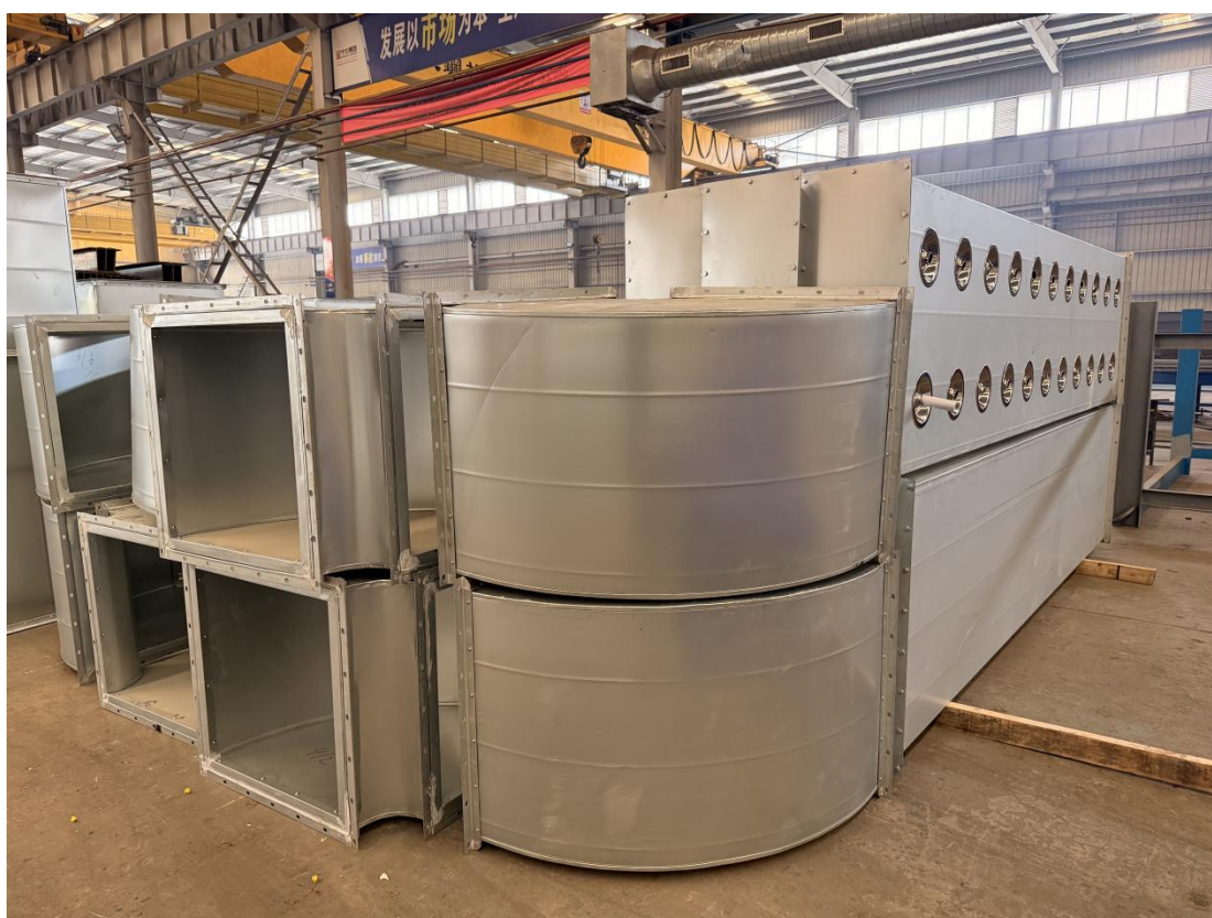
Drying room ventilation duct
