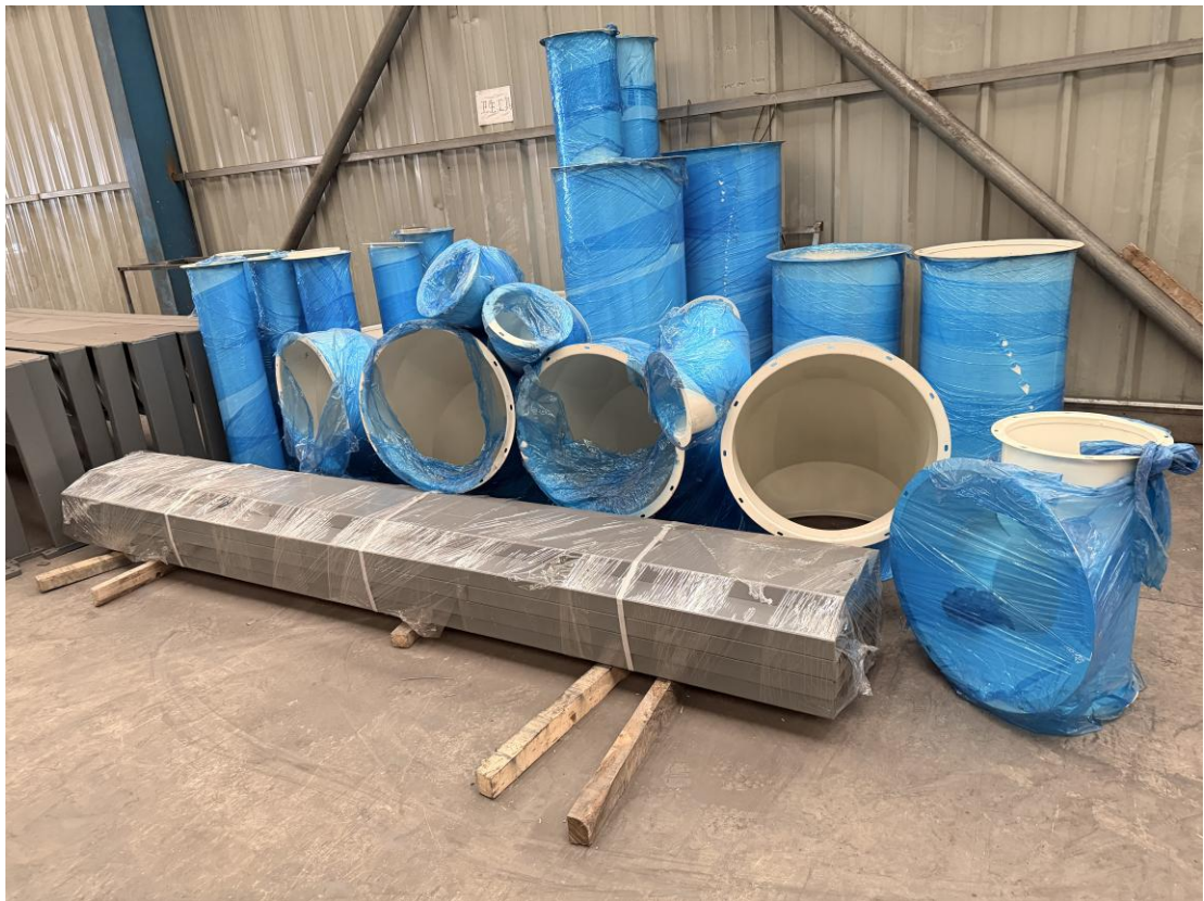
Dust removal duct
