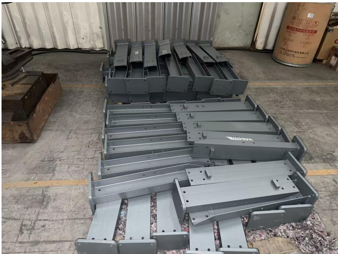
Conveyor frame support column
