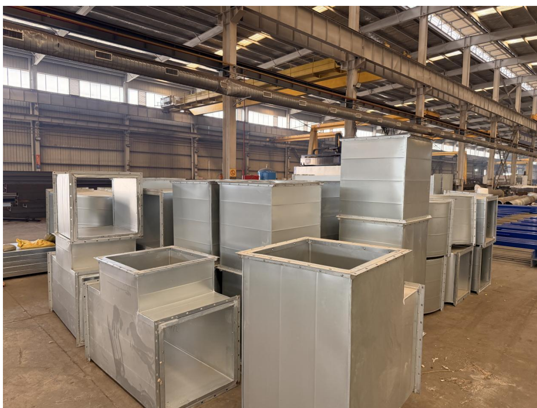
Drying room ventilation duct
