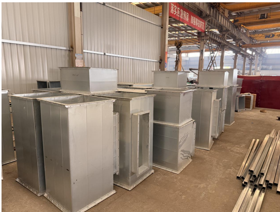
Drying room ventilation duct
